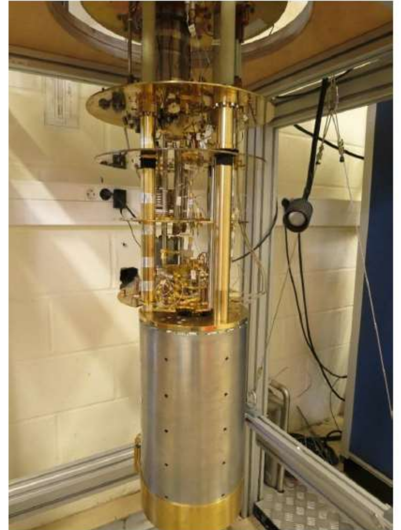
14 Tesla Dry Magnet 13mK base temperature
